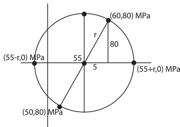
Therefore the radius of Mohr's circle is  $\sqrt{5^2 + 80^2} = 80.16$  MPa, the maximum shear stress is equal to the radius and the principal stresses are  $55 \pm 80.16$  MPa.
