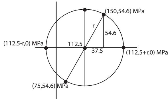
So the radius is 66.2 MPa and therefore the principal stresses are 178.7, 46.3 and 0 MPa.
