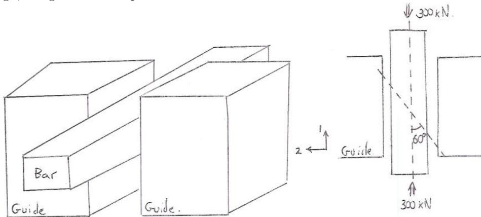
Calculate the restraining force imparted by the guides when the axial load is  $300\text{ kN}$ , given that the Young's modulus of the steel is  $200\text{ GPa}$  and that its Poisson's ratio is  $0.3$ . Therefore write down the stress matrix. Draw Mohr's circle of stress and therefore calculate the normal and shear stress on a plane inclined at  $60^\circ$  to the horizontal axis of the bar.
