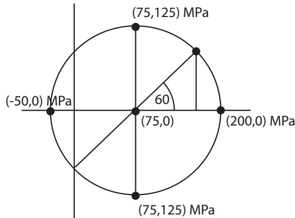
So we can write down the stress matrix for maximum shear:  $\sigma = \begin{pmatrix} 75 & 125 \\ 125 & 75 \end{pmatrix}$  MPa. These are at  $90^\circ$  to the principal axes in Mohr's circle, so they are at  $45^\circ$  to the principal axes in real space.
