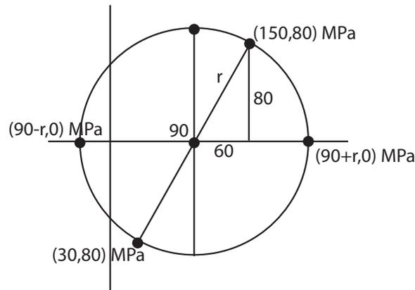
Therefore the radius of Mohr's circle is  $\sqrt{60^2 + 80^2} = 100$  MPa (3-4-5 triangle), the maximum shear stress is equal to the radius and the principal stresses are  $90 \pm 100$  MPa.
