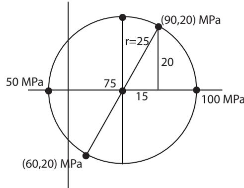
The max shear stress is 25 MPa and the principal stresses are 100, 50 and 0 MPa.
