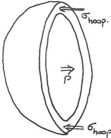
Whichever way you take the section, the hoop stresses will be the same. By inspection, we can deduce that the shear stress will be zero, and because the wall can be assumed to be thin, the radial stress will be zero. Therefore write down a stress matrix describing the state of stress in the vessel.
